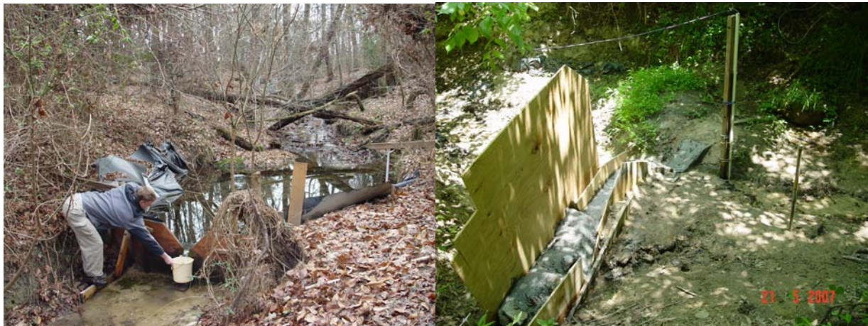
Figure 5a. Temporary (2005) and cement weirs (2007) used to measure flow in this intermittent flashy stream. The temporary weir was destroyed by flooding in June 2006. Rebar was cemented into holes drilled into the rock outcrop. The measured stage discharge curve fit well with the HEC-RAS model results
